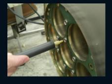
The LWL-Series Rocket Launcher Test Kit is a portable unit that tests the functionality and reliability of rocket launchers that are in service. The kit tests the electrical system of rocket launchers to ensure that they will fire rockets safely and successfully under combat conditions. The LWL-Series Test Kit can be used to test the following lightweight rocket launchers:
